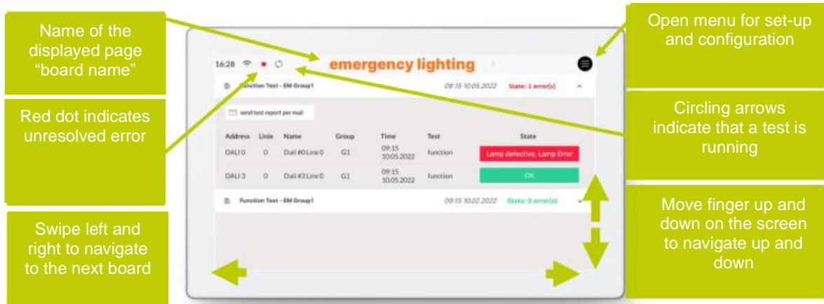
Figure 4. User Interface for Light Control DALI Display 7" Emergency. DALI system set-up and configuration see page 8. Test schedules see page 11. User interface see page 13 and following
